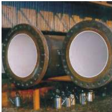
Pipes with corocoating
