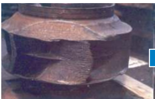
Non Coated Impeller After 4 years in a typical application
